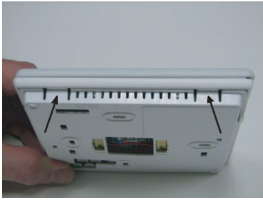
Fig. 4 - Press Tabs to Remove Backplate
